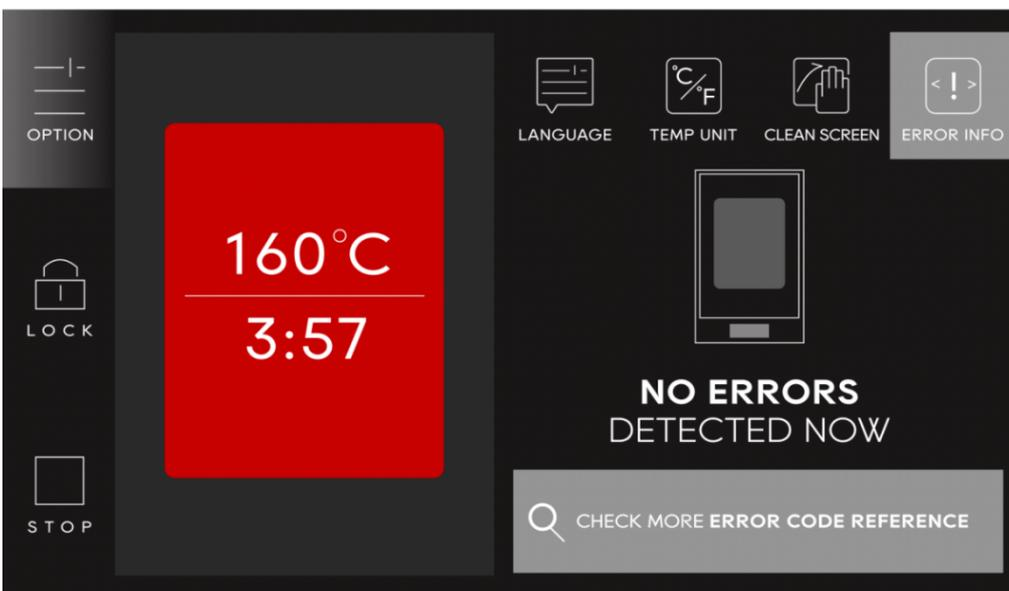
If no errors are detected, you can check the reference information via [ OPTION - ERROR INFO ].
