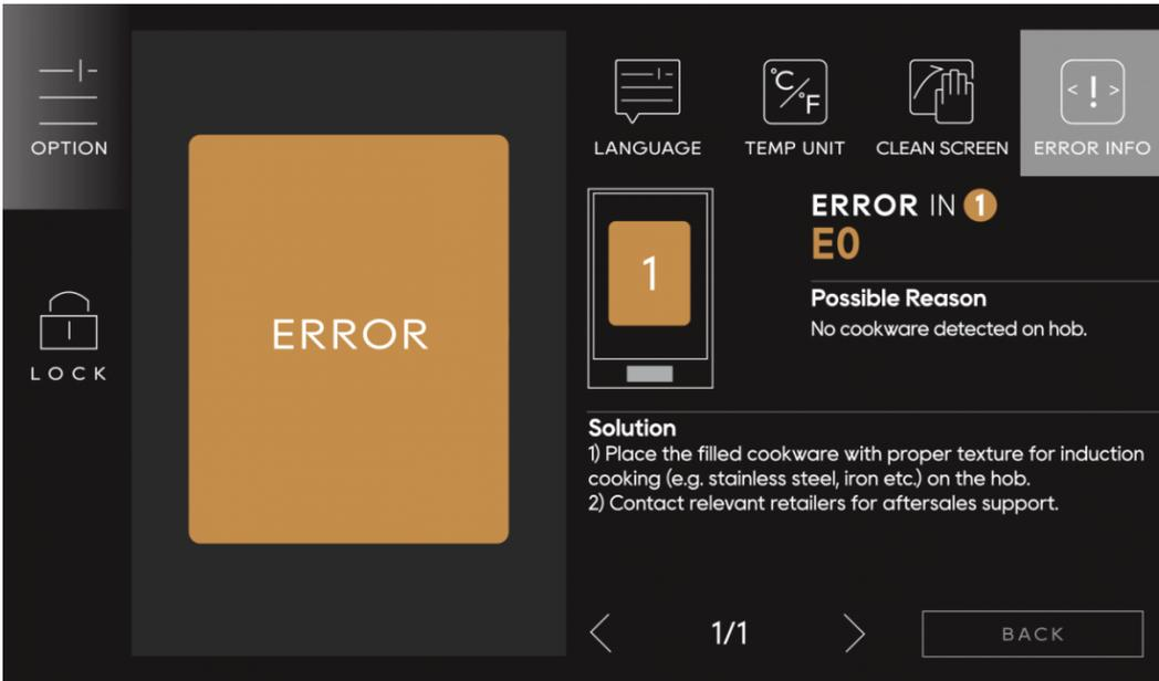
If any error is detected, you can press the lower right button to check the details.
