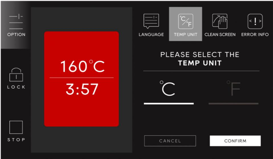
It is possible to activate the TEMP measurement unit [ OPTION > TEMP UNIT ].
