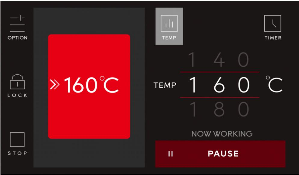
By pressing the cooking zone, in setting mode, you can press the lower right PAUSE button to interrupt the work.
