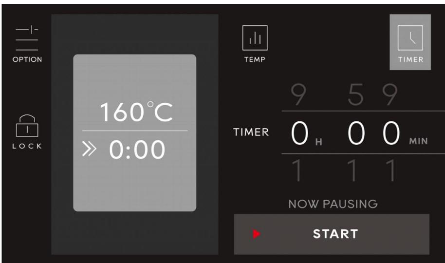
When you set POWER or TEMP for a cooking zone, you can press the TIMER icon in the upper right corner to activate the TIMER options. Set the value you want to help the product work with [POWER + TIMER] or [TEMP + TIMER] routines.
