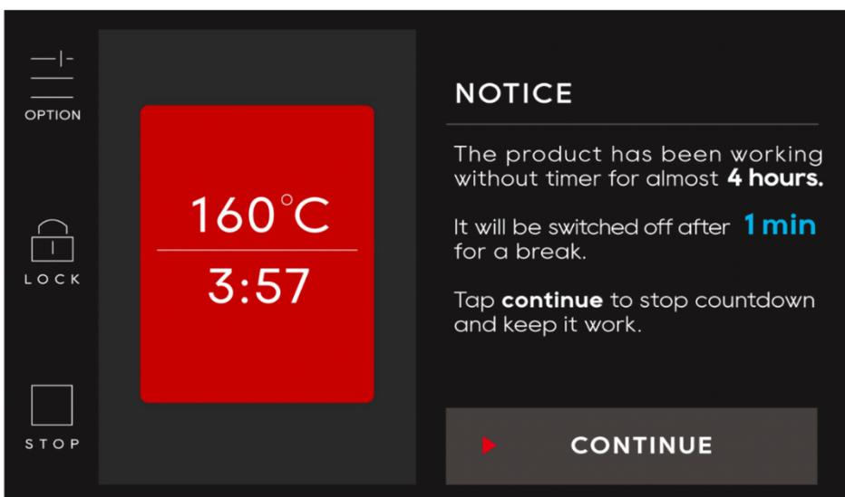
After 4 hours of operation, for safety reasons, the product starts counting down 5 minutes to activate the safe shutdown. During the 5-minute countdown, if you perform an action on the screen, the countdown will stop and the machine will resume normal operation.
